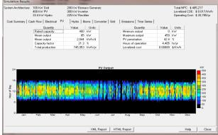
Figure 6 PV out put off grid
